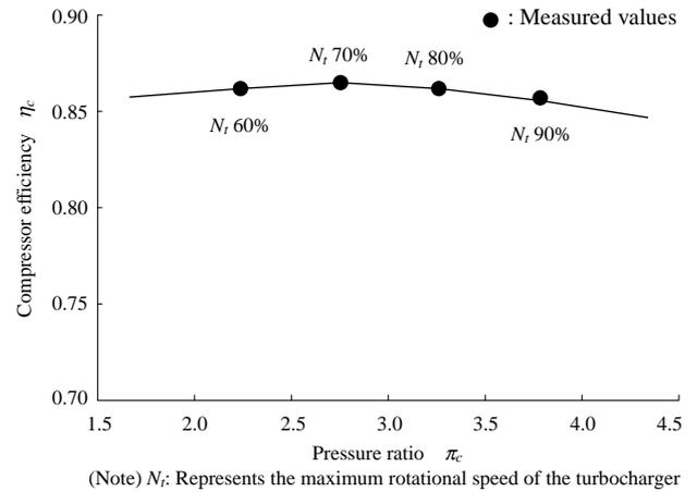
**Fig. 11 Compressor performance test results**
