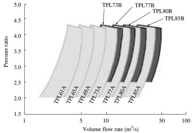
**Fig. 5** Volume flow rate ranges and pressure ratios of TPL-A and TPL-B
