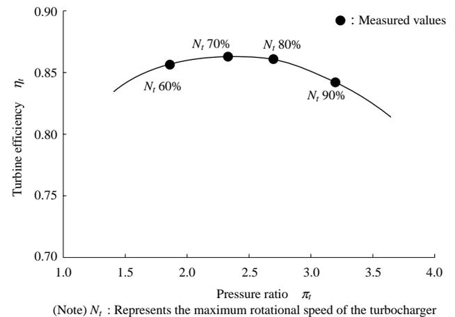
**Fig. 12 Turbine performance test results**
