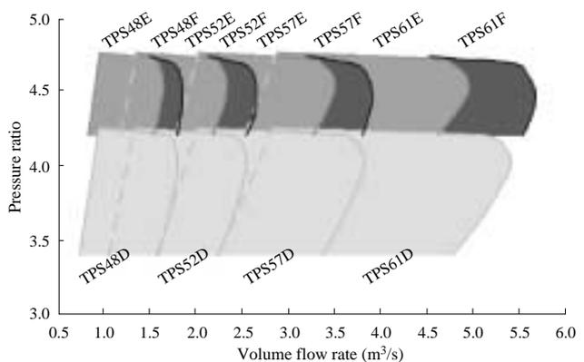
Fig. 10 Volume flow rate ranges and pressure ratios of the TPS-D, TPS-E, and TPS-F
