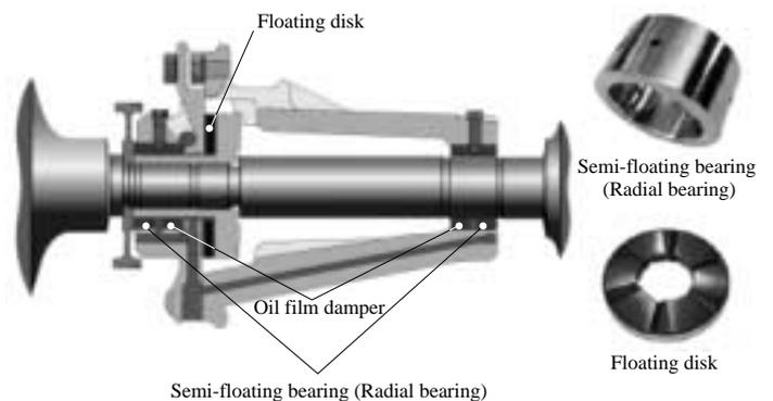
**Fig. 7** Structure of the TPL bearing
