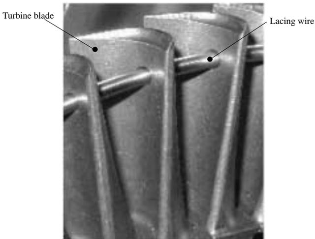
**Fig. 3** Turbine blades and lacing wire
