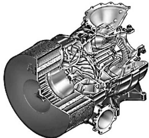
Fig. 1 Bird's eye view of the TPL-A turbocharger
