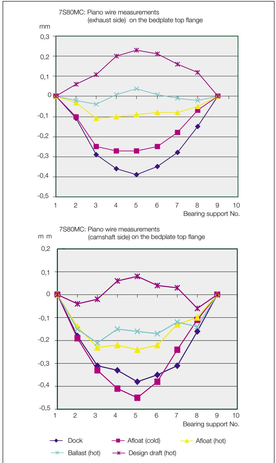
Fig. 3: Bedplate alignment for 7S80MC for VLCC
