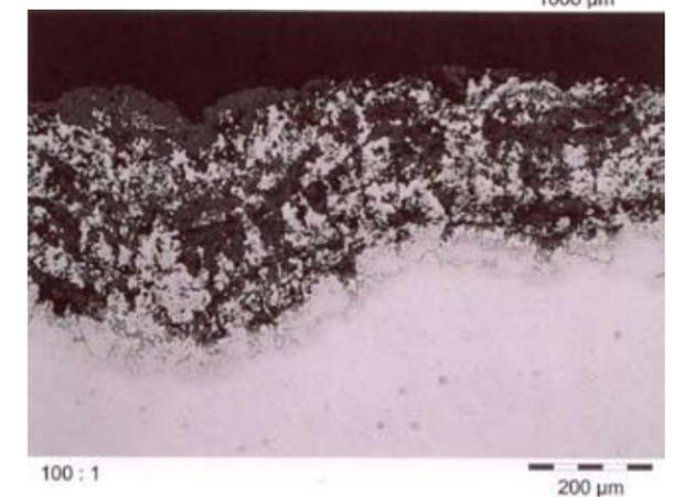
Figure 09: Micro cuts of Nimonic with high-temperature corrosion.
