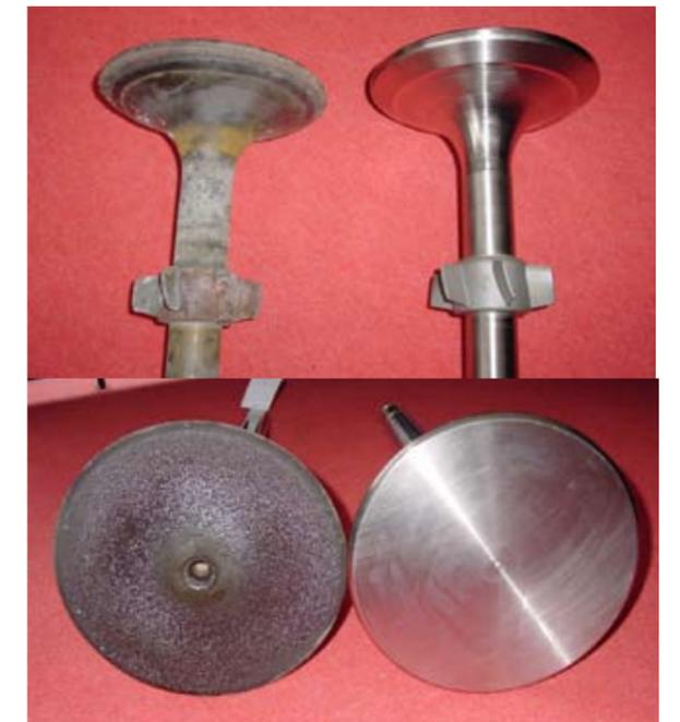
Figure 15 a/b: Nimalike spindle before and after remanufacturing
