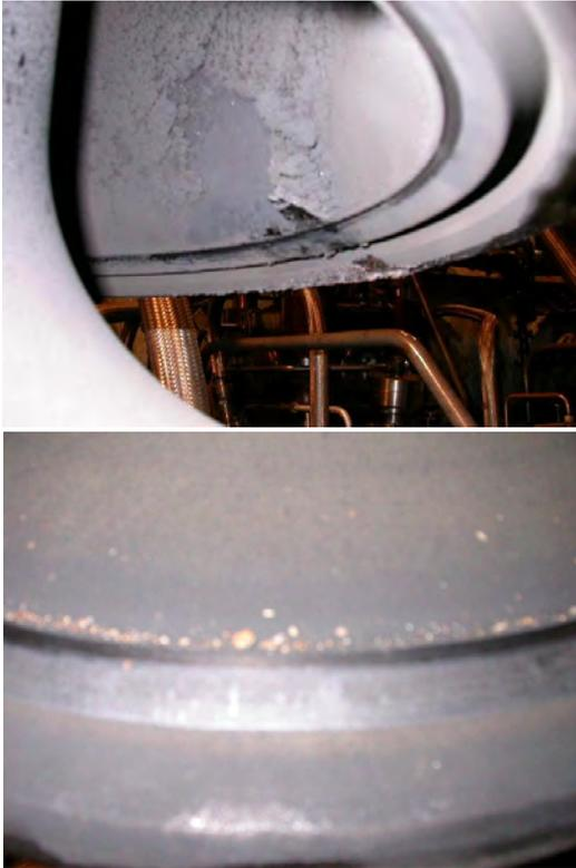
Figure 10: Photographs of the valve spindle and seat ring surfaces after 1,000 hours [6].
