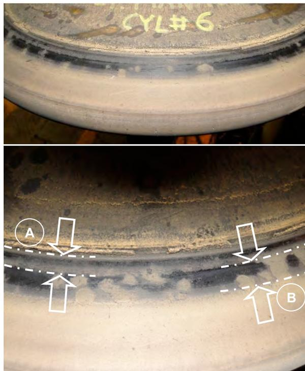
**Figure 20: Valve spindle seat with removed glassy-deposits (chamber type geometrie of bottom piece with modified seat angle for higher seating pressure).**
