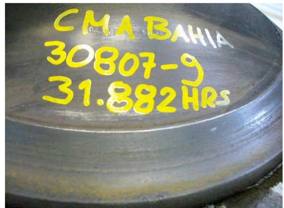
Figure 13: Photograph of valve spindle seat surfaces after 31,882 hours.
