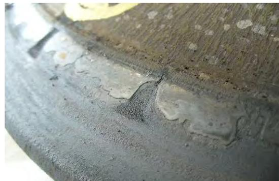
**Figure 4: Valve spindle with extensive "glassy-deposits" and beginning of blow-byes.**
