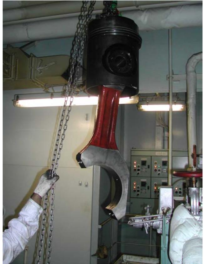
Fig. 7: Piston with new rings ready for installation
