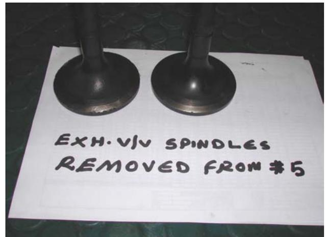
Fig. 3: Exhaust valve spindles
