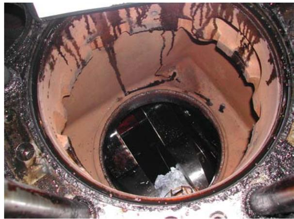
Fig. 9: Cooling water space – liner removed
