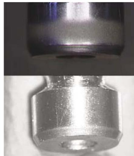
Fig. 16: Optimized design of control valve without cavitation and wear marks
