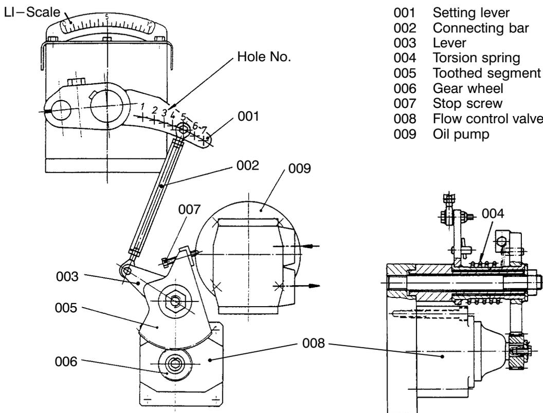
In order to guarantee an accurate cylinder lubricating oil consumption, the speed characteristics of the hydraulic motor must be correctly adjusted.
