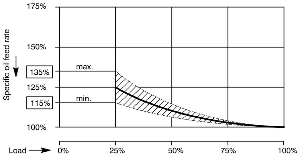
With the aid of the NOMOGRAM the specific oil delivery at 25% load must be compared to that at 100% load.
