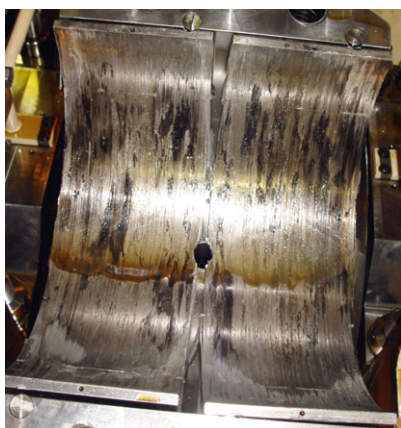
Bearing metal worn out, steel-steel contact
